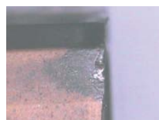
Insert of company A after 48 minutes machining
