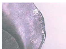
ZCC·CT insert after 80 minutes machining
